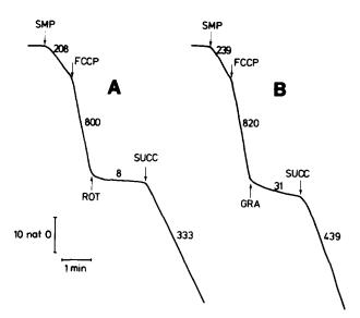
Fig. 2. Comparison of the effects of gramine and rotenone on electron transport in SMP from bovine heart. Basal electron transport was obtained by addition of SMP (0.5 mg protein) to the reaction medium containing 1 mM NADH. The uncoupled state was obtained by addition of 2.5  $\mu$ M FCCP. Other conditions were: ROT 3.5  $\mu$ M rotenone; GRA 9 mM gramine; and SUCC 10 mM succinate. Numerals on the slopes represent oxygen consumption in nat oxygen/min/mg protein.
